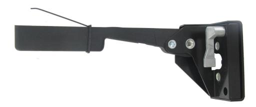
The compact 050-7130 10mm Single Rotor Latch with Squeeze Release is designed for operator door applications for off-highway vehicles that require a remote interior release. Similar to the 050-7120, this 10mm Single Rotor Latch with Direct Squeeze Release allows inside squeeze release integration into the customers door tubing.
